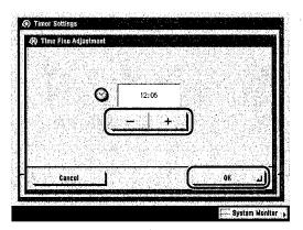
The current time is displayed in 24-hour notation, and can be adjusted in one minute increments.
