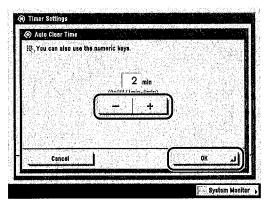
The Auto Clear Time can be set from 0 to 9 minutes (in one minute increments).
