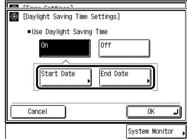
Set the month, week, day, time to start and end the Daylight Saving Time settings, and press the [OK] key.
